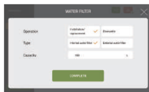
5.Select installation/replacement and internal water filter, input water capacity based on suitable level,then touch complete
